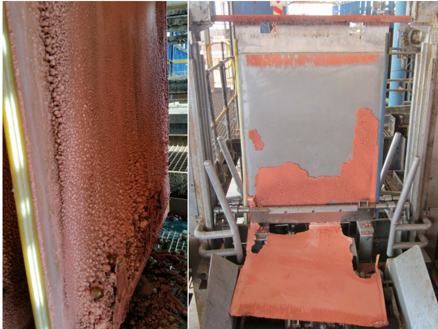
Figure 1: Severe nodulation resulting in impure copper and, in extreme cases, brittle copper which breaks up during stripping
