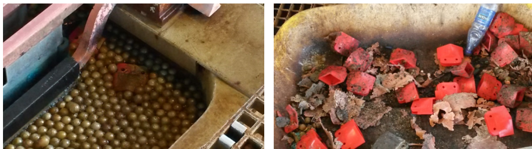
Figure 2: Dislodged and damaged anode spacers.
